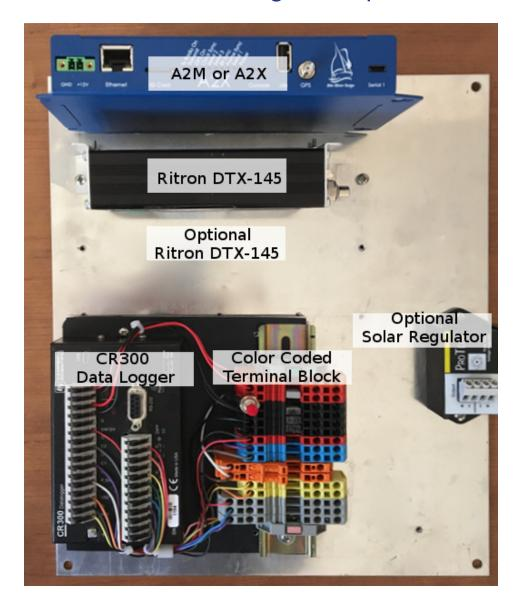
Image showing the layout of Blue Water Design's flexible backplane. Dimensions are 10.88" x 12.75". Cables are not shown for clarity.
